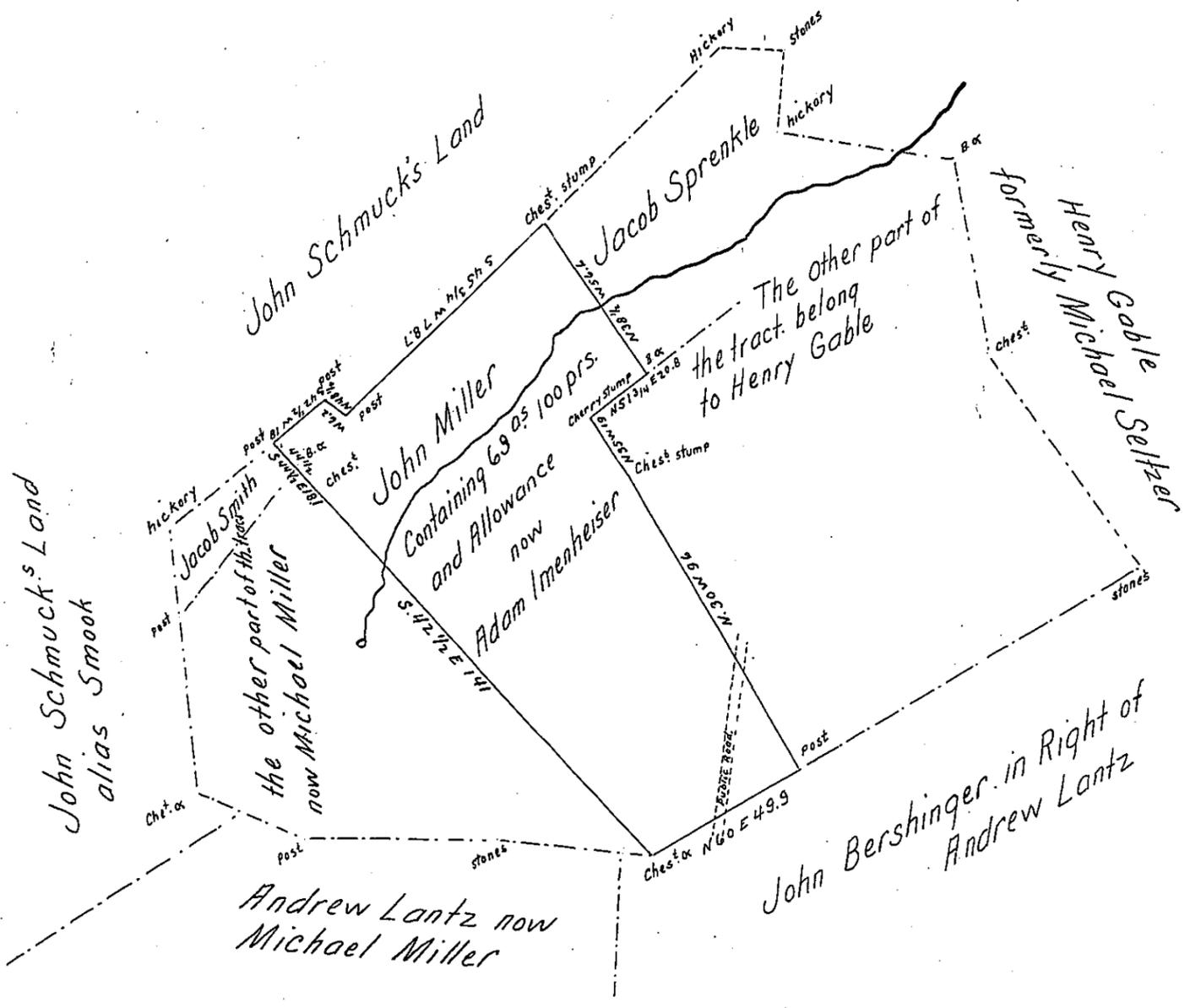
A Draught of a Piece of Land Situate in Windsor Township in the County of York. Containing as above set forth 69<sup>as</sup> 100<sup>prs.</sup> and allowances &c. which is part of 236<sup>as</sup> 13<sup>prs.</sup> and allowances &c. Which was Originally Surveyed On the 19<sup>th</sup> of the 10<sup>th</sup> Month 1768. for John Miller in purs-
